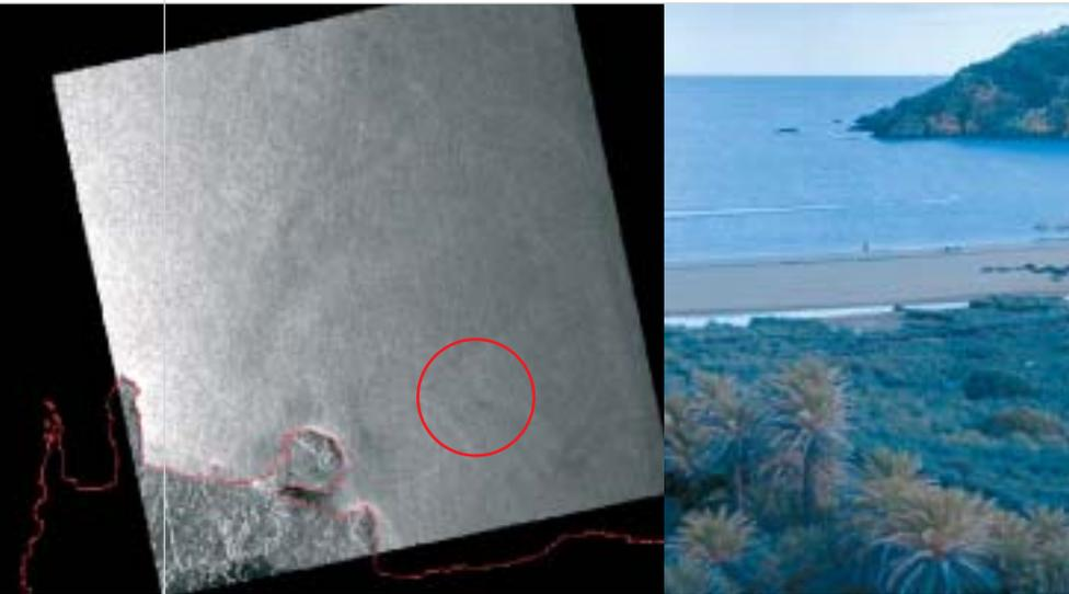
*To fight oil pollution, the PROMED project is based on the development of the synthetic aperture radar imaging and very high resolution radiometry. Circle on left picture indicates the location of a possible oil slick.*
